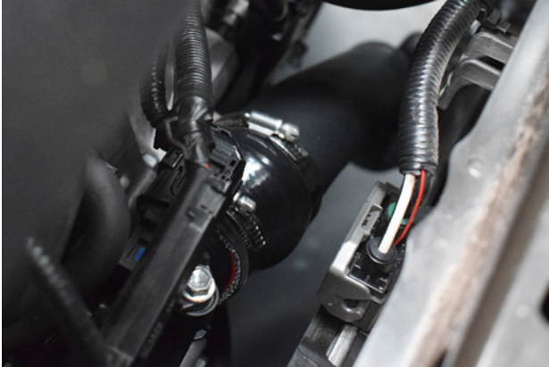
37. Install the silicone reducer followed by the hardpipe 'without' the honeycomb bracket.
