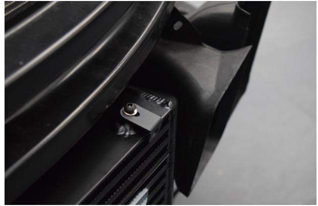
50. Install the small L bracket on top of the intercooler using the supplied screw and washer.
