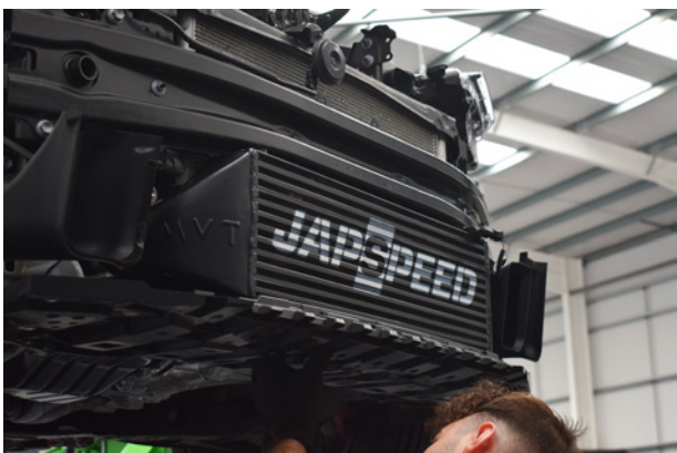
53. Install the tray under the intercooler.
