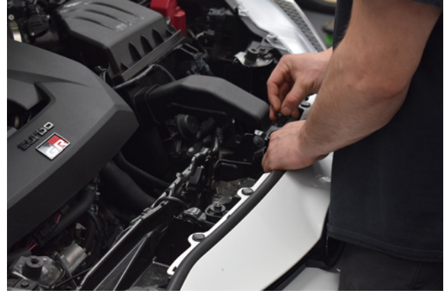
2. Remove the 2x outer push clips across the top edge of the bumper.
