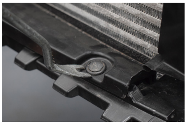
18. Remove the clips on the plastic tray under the intercooler.
