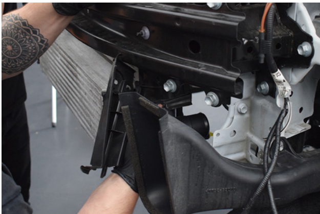
21. Remove additional plastic trim, these will not be fitted with the new intercooler.
