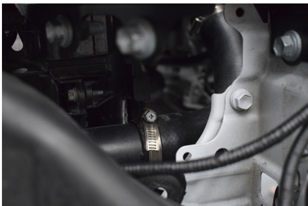
23. Undo the clamp on the intercooler outlet pipe using a socket or screwdriver.
