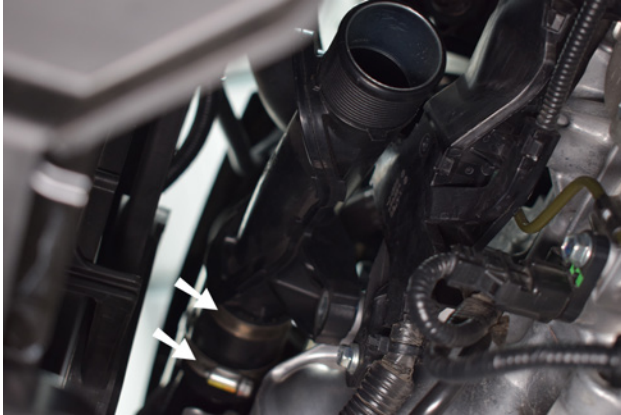
25. Undo the 2x clamps and bolt from the pipe bracket and remove from the throttle body.
