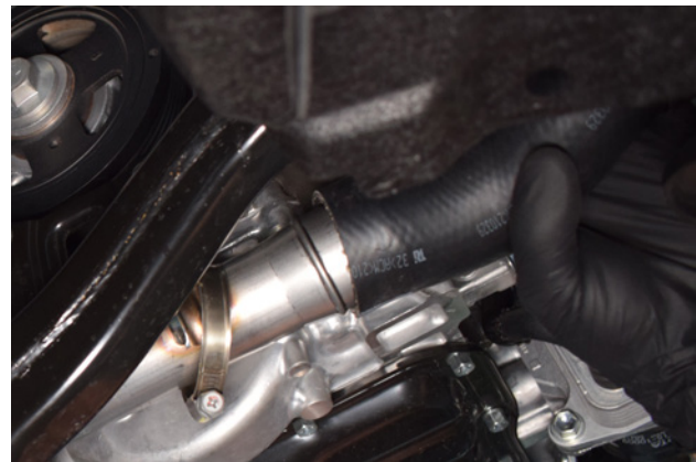
28. Remove the silicone pipe.
