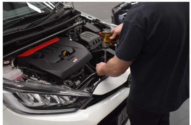
58. Install the 2x 10mm bolts on the top of bumper along with the 2x trim clips.
