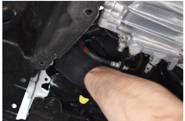
40. Install the 90° silicone pipe.
