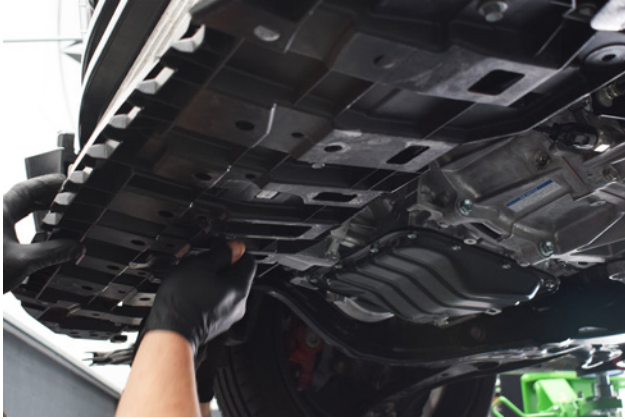
19. Remove bolts from the underside of the intercooler tray.
