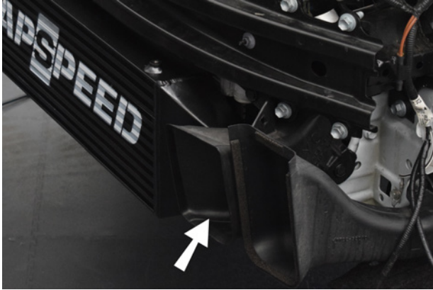
49. Install the cooling duct and re-insert mounting clips.
