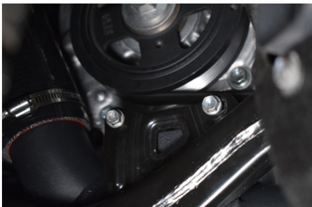
48. Secure the hardpipe bracket using factory hardware and tighten all clamps.
