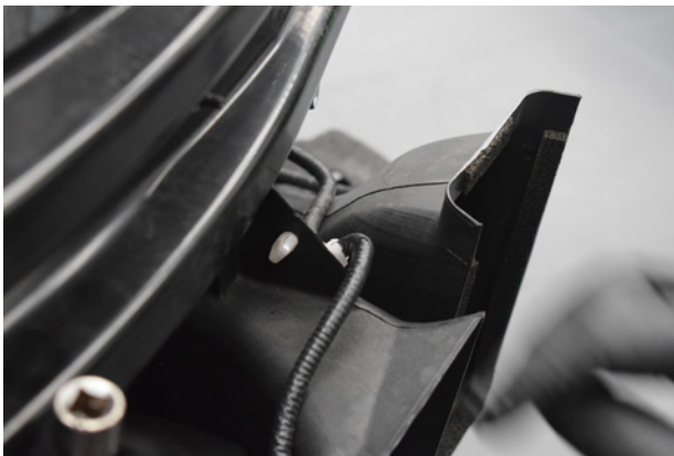
51. Clip sensor wiring back into the cooling duct.
