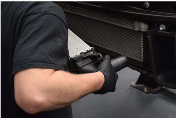
33. Carefully remove the intercooler.
