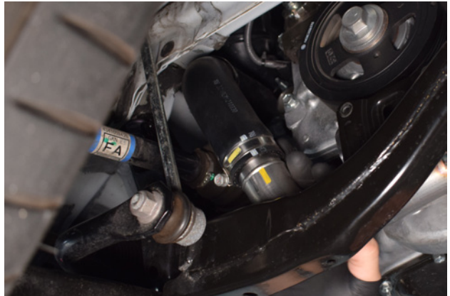
30. Remove 2x bolts securing the hardpipe and remove remaining pipework.
