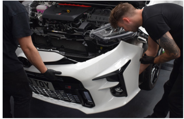
56. Install the front bumper, remembering to re-connect the fog lights.
