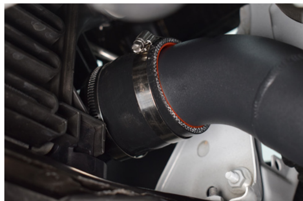
47. Place the straight silicone pipe on the hard pipe and secure to the intercooler inlet.
