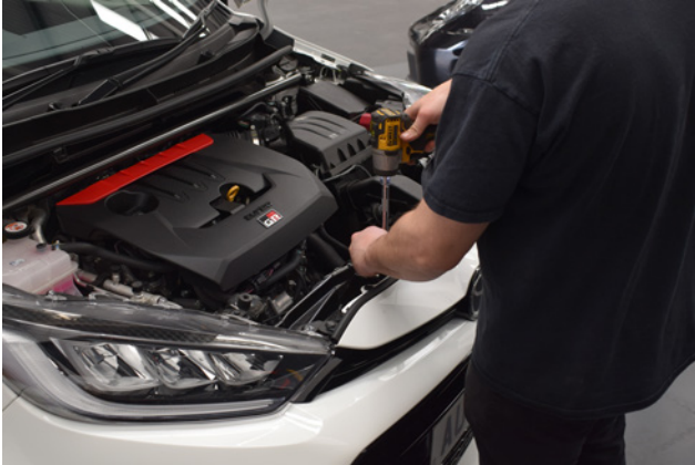
1. Remove 2x 10mm bolts located on the top of the bumper.
