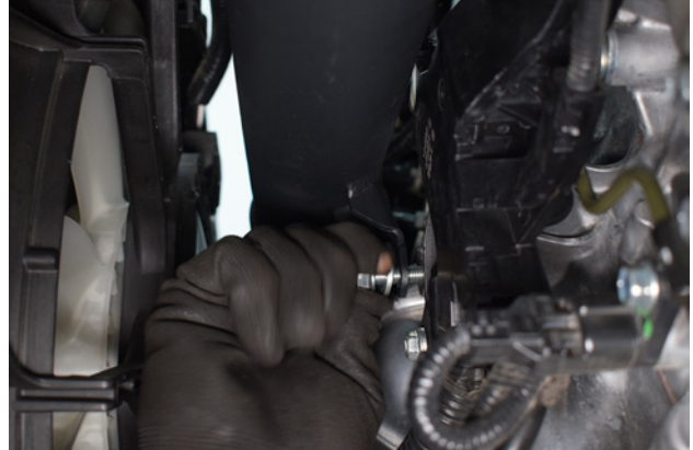
38. Secure the hardpipe bracket using the factory hardware.
