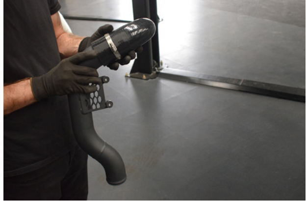
44. Place the second 90° silicone which reduces to the turbo onto the remaining hardpipe.
