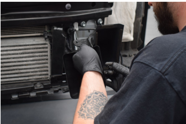
17. Remove the left hand cooling duct, this will allow access to the intercooler boost pipe clamp.
