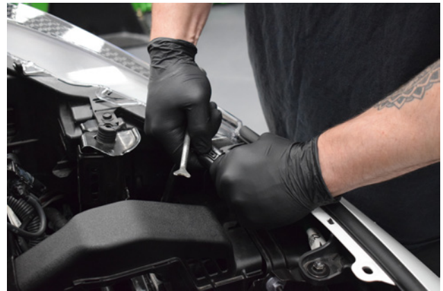
4. Undo electrical connector on the left side.
