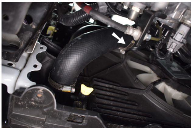
24. Undo the upper hose clamp and remove the silicone pipe.
