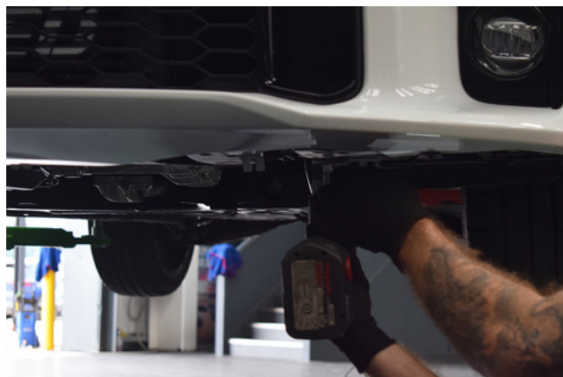
5. Remove 10x 10mm bolts from the underside of the front bumper and remove the undertray.
