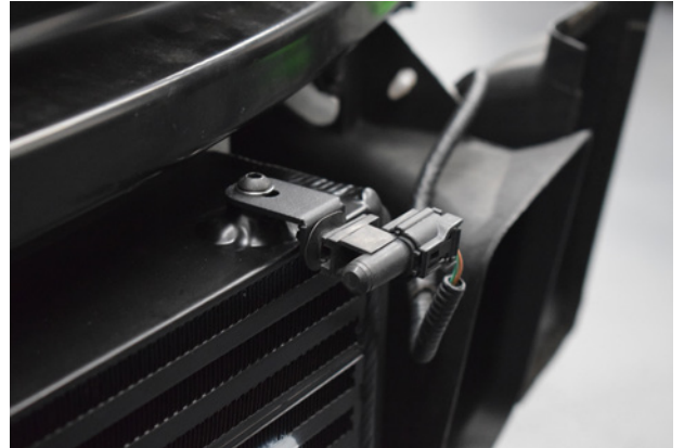
52. Clip sensor into the new bracket.
