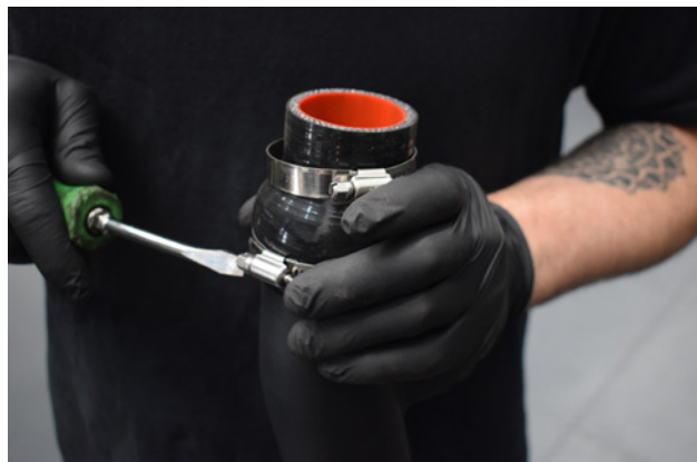
36. Prepare the silicone reducer, ready to install onto the throttle body.
