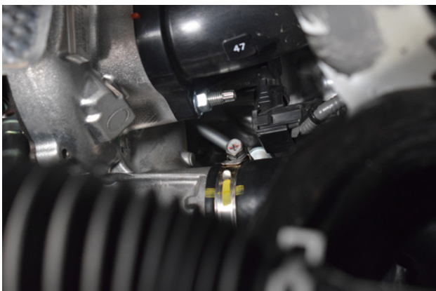
29. Undo the clamp securing the pipework to the turbo.
