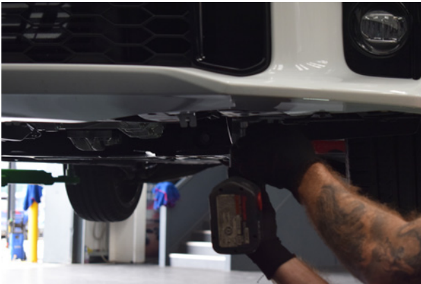
57. Install all the bolts underneath the bumper.
