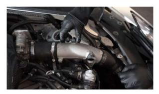
30. Remove upper boost pipes by removing clips at end.
