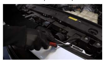
7. Unclip and remove side repeaters.
