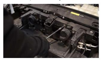
33. Remove the 10mm bolts attaching intercooler mounts to car.34. Unbolt intercoolers from mount, remove pipes and slide out.
