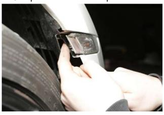
8. The bumper is attached by 2x10mm bolts located on each side. These can be reached using a long extension.
