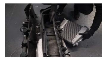
35. Remove rivets on shroud.
